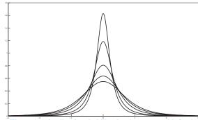
Figure 1: A family of probability density curves with fixed mean and variance, and varying skewness.
